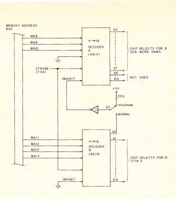
Fig. 6. Modified memory select circuit.
